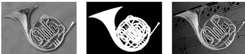
Photoshop image (left) contains an alpha channel mask (center), which Premiere uses to composite the subject against another background (right).
