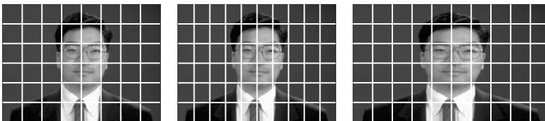
Frame with square pixels (left), frame with tall horizontal pixels (center), and center frame again displayed using square pixels (right)
